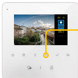
Press "Down" to switch to camera
