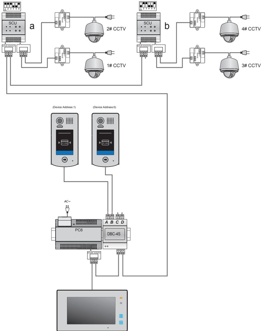
NOTE: The system can connect SC6V(SC6V connected two TYPE B Cameras), but at this time, the DIP6 of DT-SCU must be set to ON.
