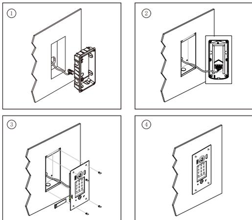
1. Drill a hole in the wall to match the size of the mounting box and attach to the wall.
