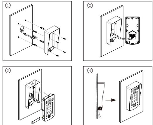
1. Drill holes in the wall to match the size of screw stoppers, then attach the rainy cover to the wall.
