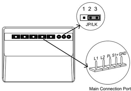
**Lock Control Jumper:** To select the lock type.
