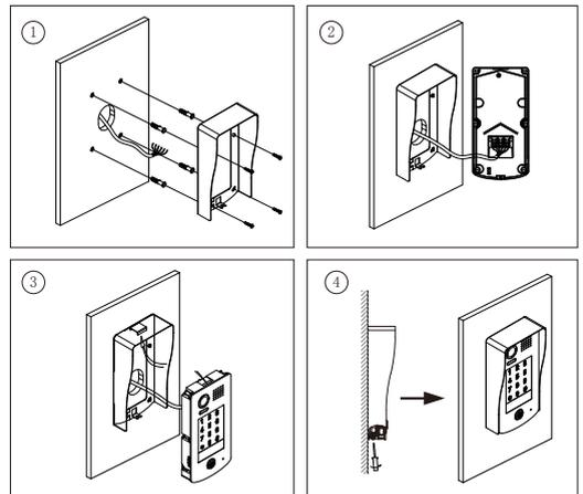
1. Drill holes in the wall to match the size of screw stoppers, then attach the rainy cover to the wall.
