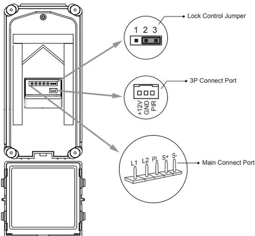
**Lock Control Jumper:** To select the lock type.
