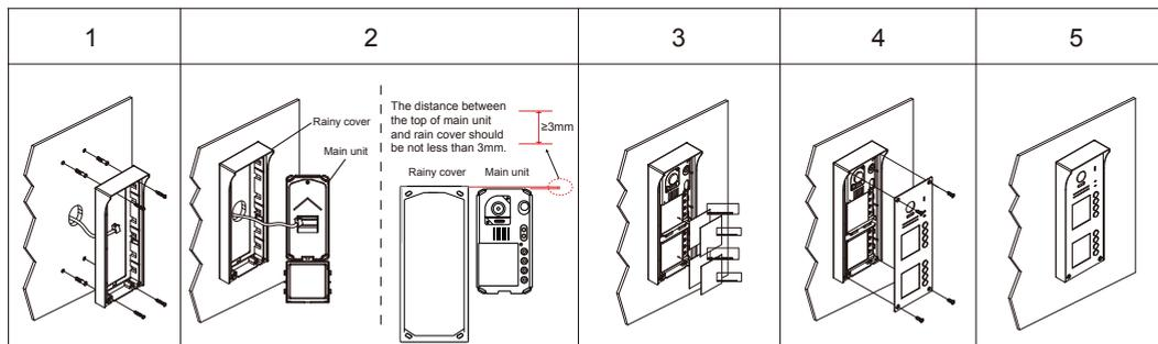
1. Drill holes in the wall to match the size of screw stoppers, then attach the rainy cover to the wall.
